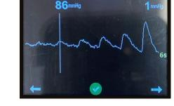
In this example, the waveform was moved to the right until the first clear waveform was determined. There is a small amount of artifact, which will not interfere with an accurate reading of the test. If no clear waveform can be found, discard the test and perform again.
